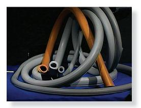
E/Insulation is a silicone hose used to protect a variety of distribution and substation equipment up to 20 kV phase-to-ground. The E/Insulation is manufactured with a split seam to allow for an easy application without the need of breaking electrical connections. The hose is simply pulled and split apart allowing it to be quickly slipped over the cable or bus being protected. There is no heat shrinking required for application and no tools other than a cutting tool for proper length are needed.
